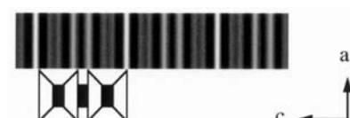
Figure 4. The lattice images of interstratified serpentine/smectite = 2/1 compound and interstratified chlorite/smectite = 1/1 mineral simulated by MacHREM under the condition of defocus = 870 Å. All of them are polytypism consisting of 4 tetrahedral sheets and 3 octahedral sheets.
